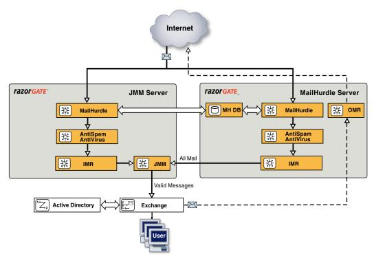
Figure 5 RazorGate Scenario with JMM and Active Directory with Exchange
