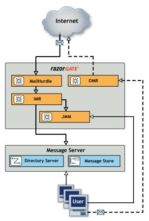
Figure 13 JMM Combined with the IMR Tier
