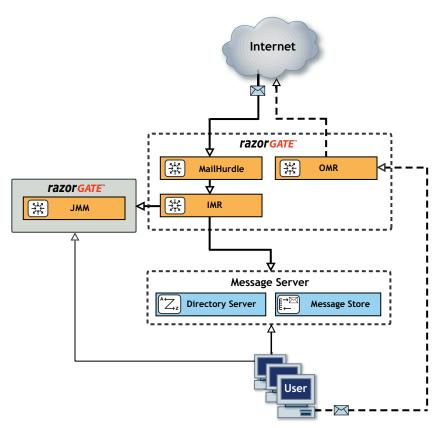
Figure 14 Splitting JMM and the IMR
