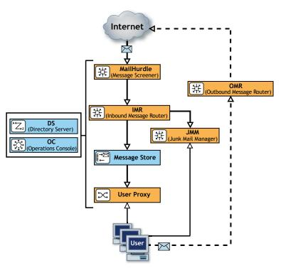
Figure 2 Mirapoint Security and Messaging Functions
